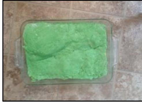
Figure 12. Non-conductive 'waste rock' is added to fill the rest of the container.
