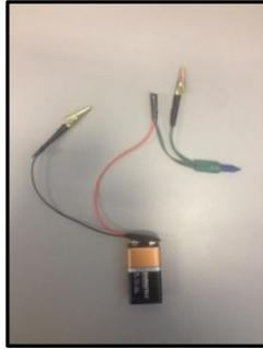
Figure 4. Assembled conductivity meter (option 1).
