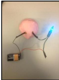
Figure 5. Conductivity meter on conductive play-dough.
