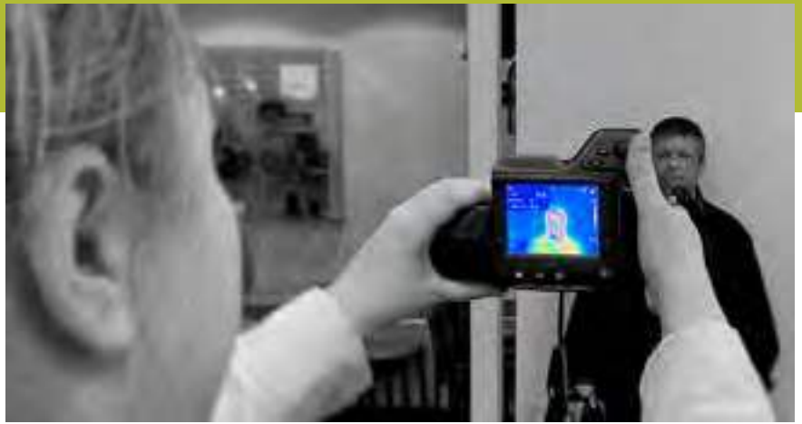
Thermography camera scans employee for increased temperature. Photo courtesy of Cameco Corporation.
