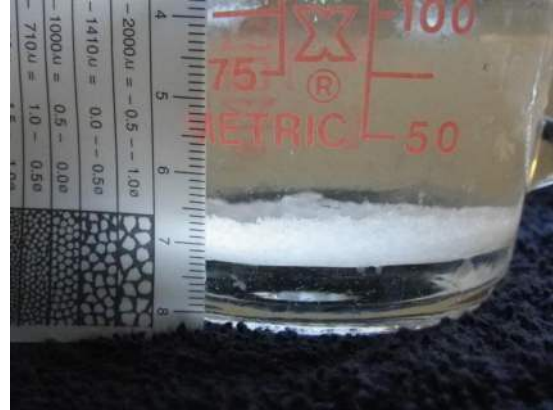
A layer of potash crystalline mush has formed on the bottom of the measuring cup.
